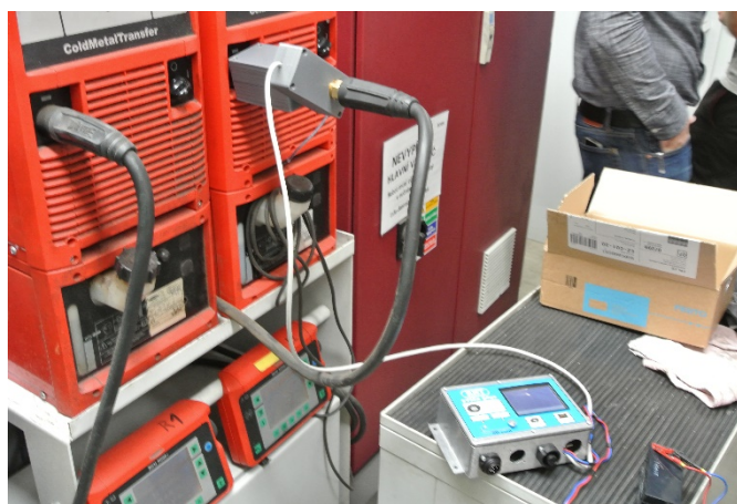
Figure 3 - Connected HSCSS. The processing unit is equipped with small touch-panel for operator.
