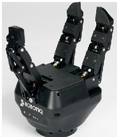
Fig. 8 Example of adaptive multijoint gripper inspired by bionic (Robotiq) [12]
