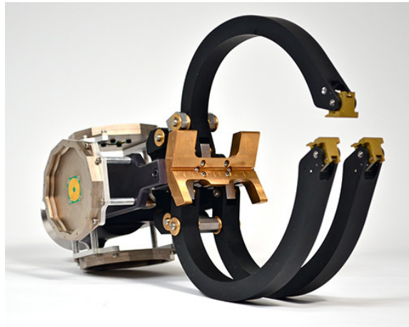
Fig. 7 Example of wide-range gripper (Universal Gripper Anchor, Honeybee Robotics) [11]
