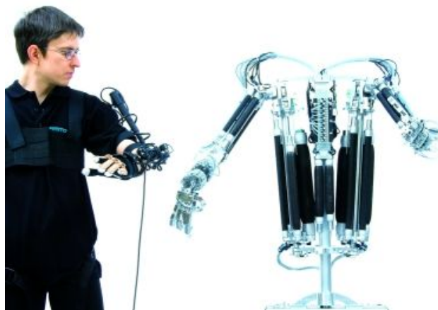
Figure 7 – Based on pneumatic artificial muscles (fluidic) Festo has launched a joint venture project by EvoLogics GmbH and the Faculty of bionics and evolution of technology of Technical University of Berlin.
