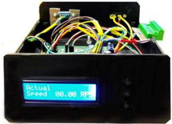
Fig. 3. Opened control unit
