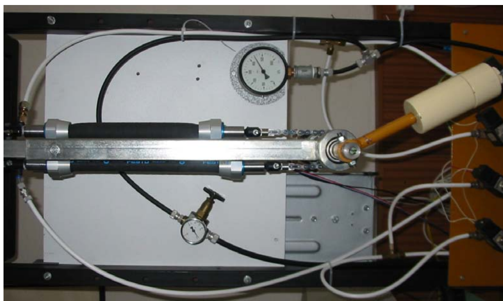
Figure 1 – Pneumatic actuator with artificial muscles
