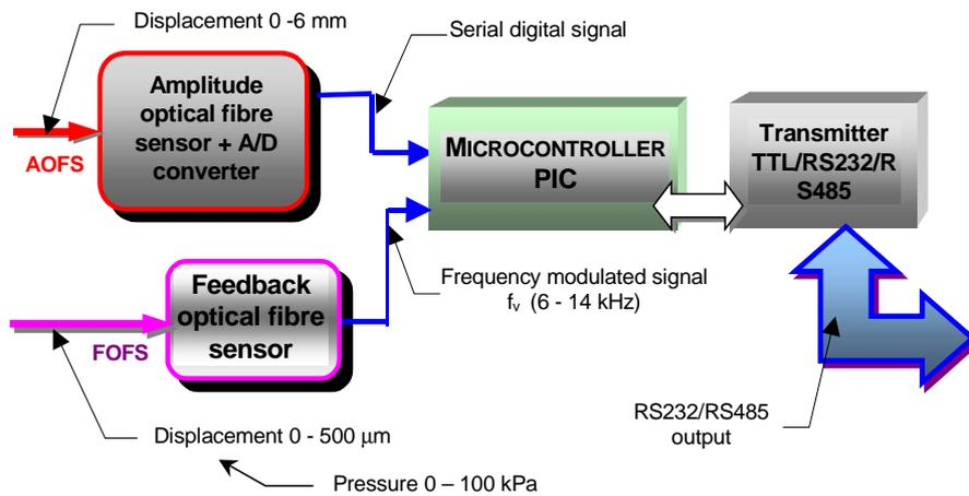
Fig. 4 Block schema of two optical fibre transducers connected to the Smart displacement sensor (SDS) with digital output
