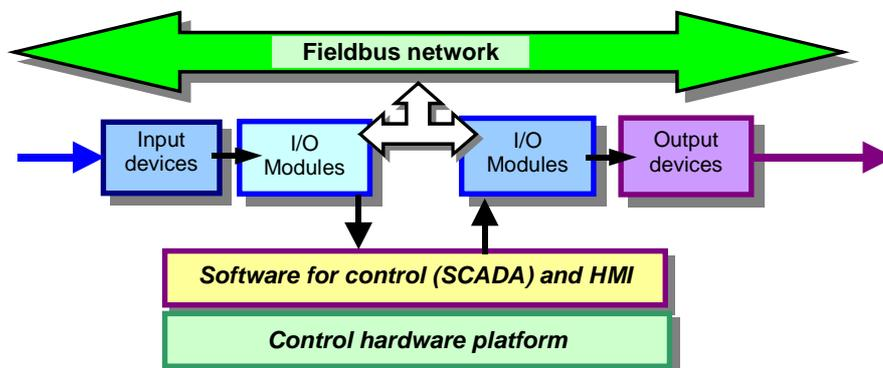
Fig.2 Today's control architecture - typical PLC structure of controllers with separating I/O modules communicating by Fieldbus network
