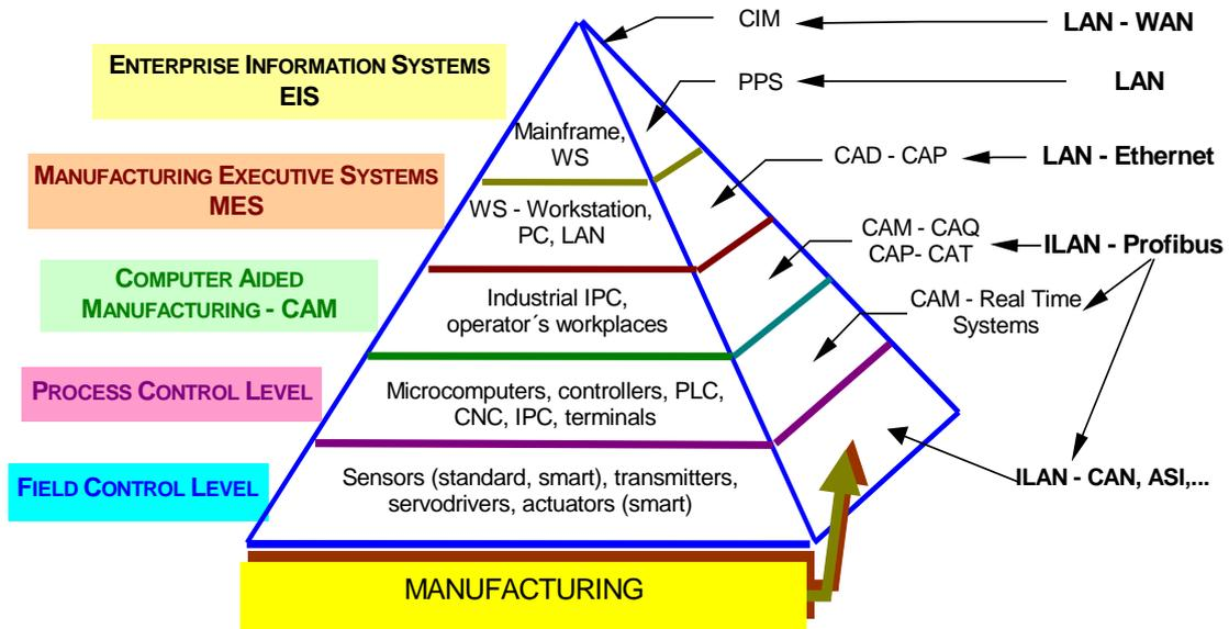
Fig. 1 Multilevel distributed control system with ILAN/LAN support
