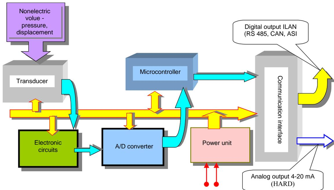
Fig.3. Block schema of SMART SENSOR connected to the Industrial LAN
