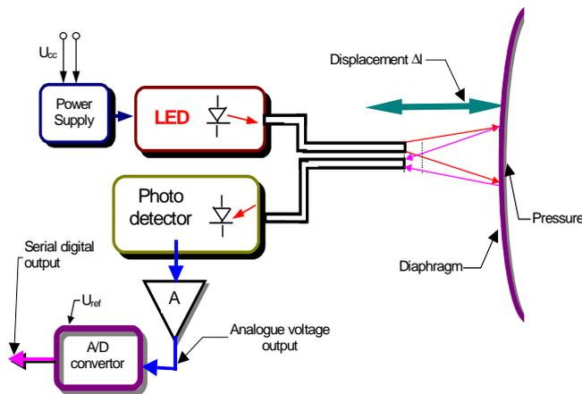
Fig. 5 Principle block schema of amplitude optical fibre pressure sensor with voltage output - AOFS
