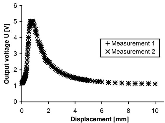
Fig. 6 Experimental characteristic of amplitude optical fiber displacement sensor with voltage output - AOFS
