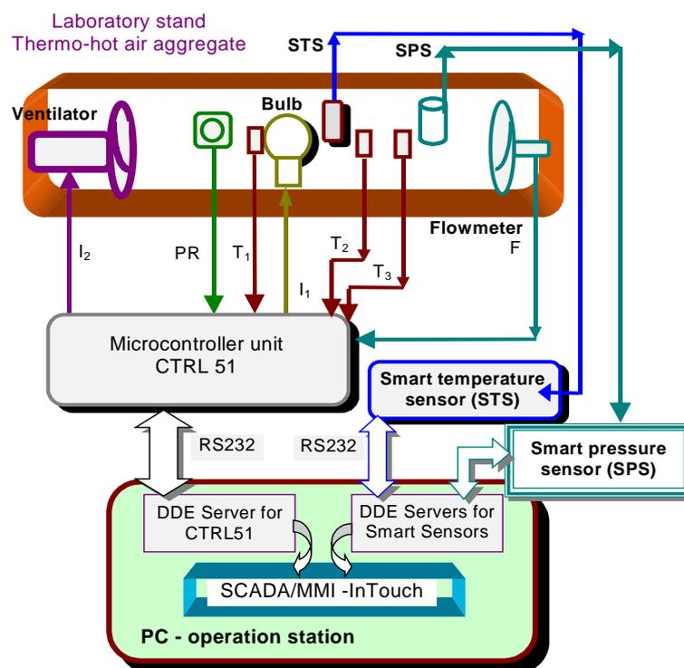
Fig. 7 Block schema of laboratory stand with CTRL 51 and smart sensors connected to PC with SCADA/MMI program system InTouch
